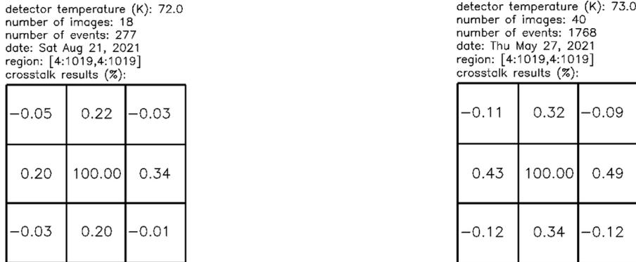
Figure 6. Crosstalk is similar for V23 (left) and F17 (right). The nearest-neighbor values are low for both devices, and somewhat lower for V23 as compared to F17.
