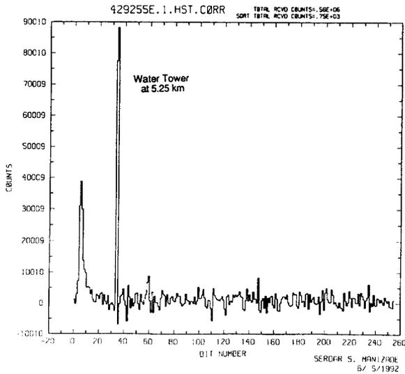
Figure 3. AlGaAs Lidar Measurements
