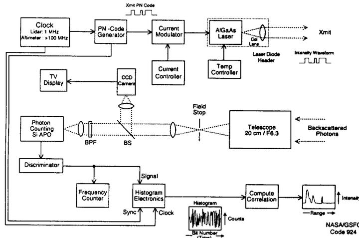
Figure 2. AlGaAs Altimetry Measurements
