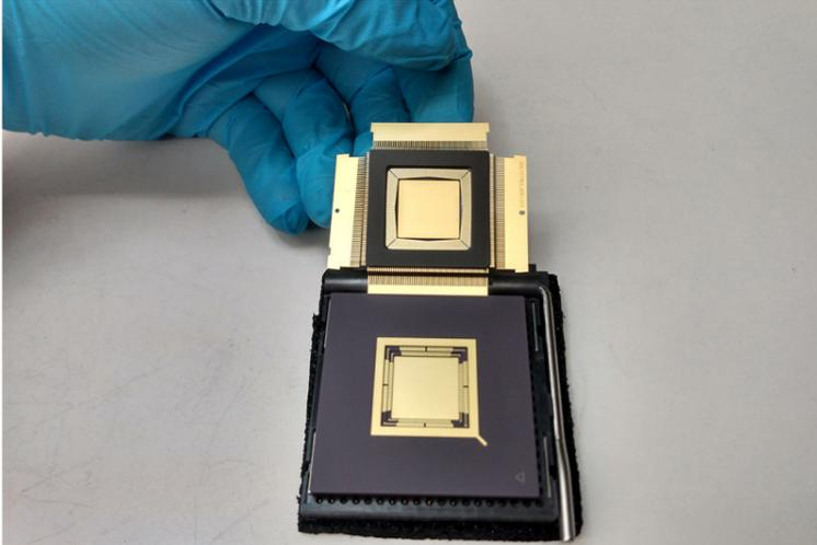
Justin Gallagher is serving as project manager for a nearly \$1 million grant funded by NASA to create a single photon sensing and number resolving detector for NASA missions. Pictured above are candidate detector chip carriers and socket ready for cryogenic testing.
