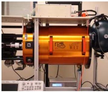
**Testing in a vacuum:** This helium-cooled vacuum device, known as a Dewar test system, will be used to determine the effectiveness of a new LIDAR system for mapping planets. LIDAR's sensors are placed in the Dewar test system to create a carefully controlled environment in which to determine their efficacy and accuracy.
