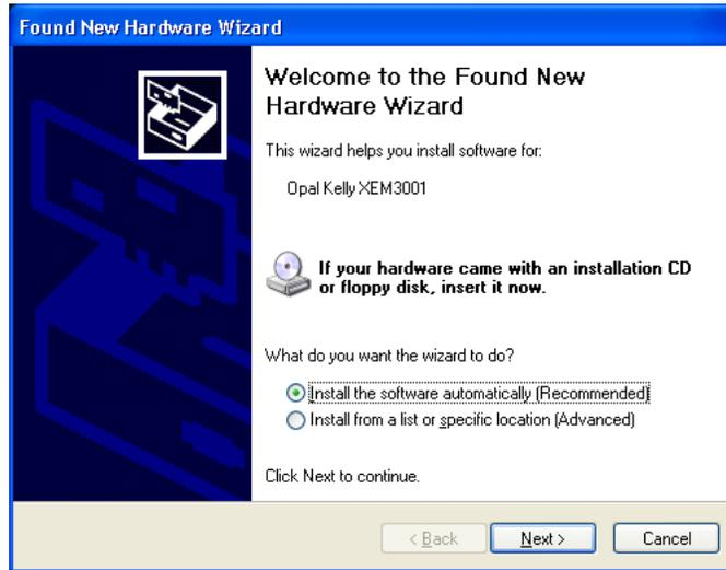
Allow Windows to install the software automatically and click **Next**. Windows should then properly locate the driver installed previously and complete the installation. Your XEM is now ready to be used and will be recognized in FrontPanel.
