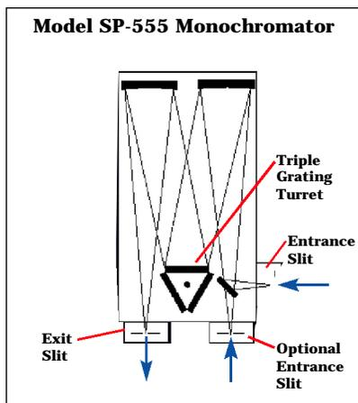
Includes 90° optical path, and micrometer adjustable entrance and exit slits.
