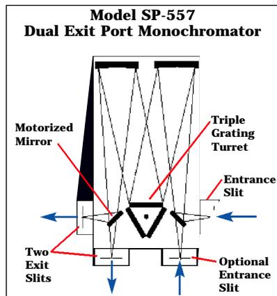
Includes micrometer controlled dual exit slits (90 & 180°), and motorized mirror for rapid, computer controlled exit slit selection.
