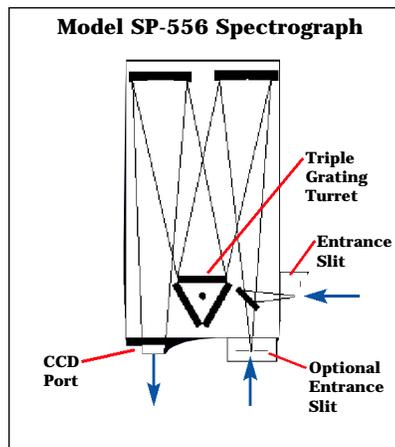
Includes 90° optical path, large 14mm X 27mm focal plane, plus sliding tube CCD adapter with focus-stop.
