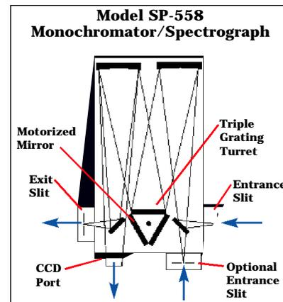
Includes dual exit ports; one exit slit and one sliding tube CCD adapter with motorized mirror for rapid, computer controlled exit port selection.
