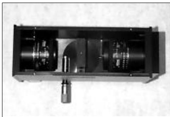
Inside view of the NFC-446-040 showing the sample holder and micrometer positioned between the collimating and focusing lenses.
