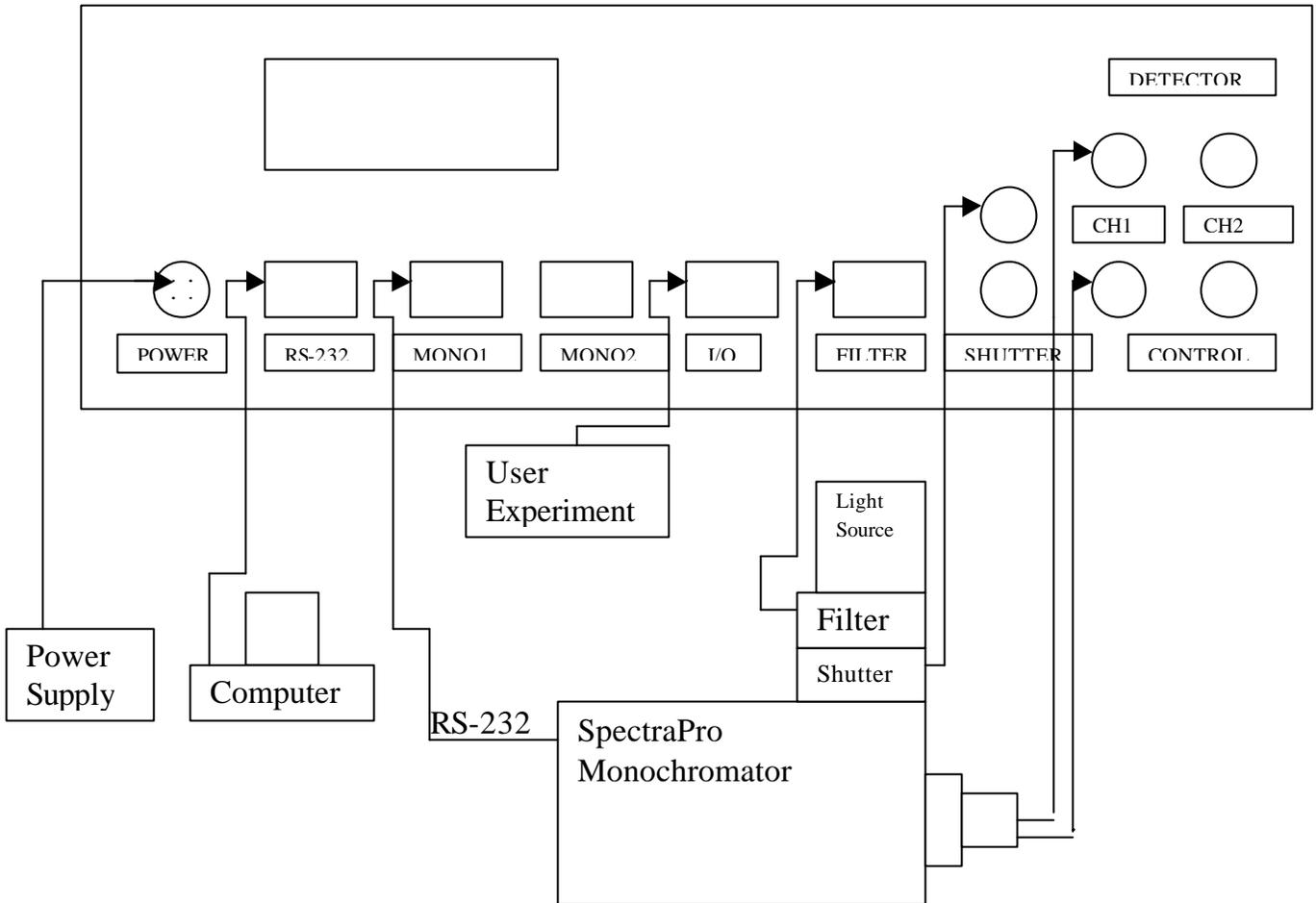
If the experiment utilizes two monochromators, the RS-232 port on the second monochromator is connected to the MONO2 port on the NCL using the serial cable supplied with the monochromator.
