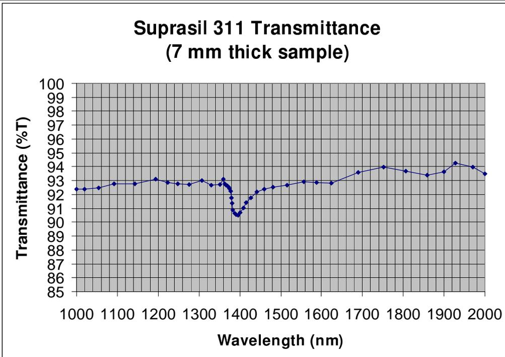
Figure 2 : transmittance of a 7 mm thick window of Suprasil without AR coating. This thickness is representative of the RCP. Notice how the increased thickness increases the depth of the water dip at 1.383  $\mu\text{m}$  without changing the overall transmittance (dominated by surface effects).
