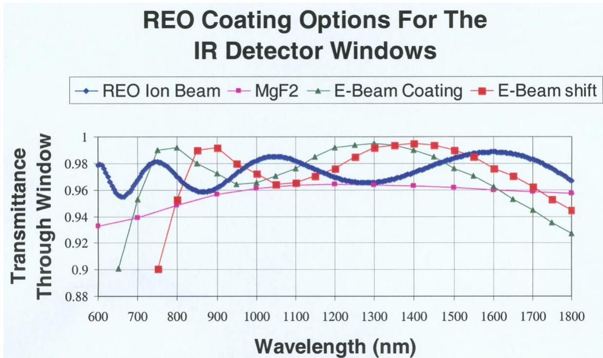
Figure 3 : transmittance as a function of wavelength of the various coating options for the IR channel window. The shifted E-beam coating (large red squares) is the best compromise between transmittance and risk.
