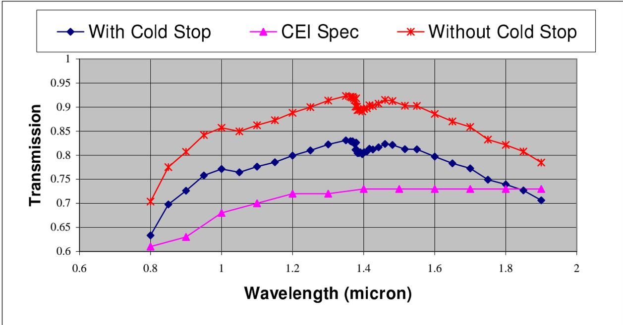
Figure 5 : predicted throughput of the WFC3 IR channel including (blue diamonds) or excluding (red crosses) the cold stop loss but excluding the OTA and the detector. The throughput remains above CEI Specifications (purple triangles) over the whole wavelength range of the instrument (0.85-1.7  $\mu\text{m}$ ).
