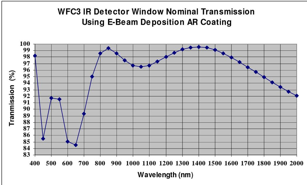
Figure 4 : shifted E-beam coating transmittance as derived from the detailed REO design model. These values are in agreement or exceed the predictions of the simple model of Figure 3.
