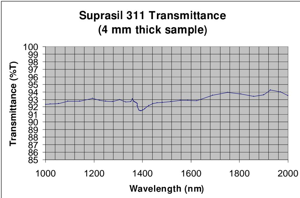
Figure 1 : transmittance of a 4 mm thick window of Suprasil 311 without AR coating. This thickness is representative of the detector window. The dip at about 1.383  $\mu\text{m}$  is due to residual water absorption in the glass.
