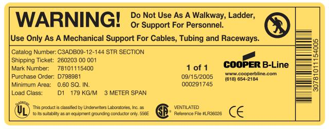
This cable tray label is attached to each straight section and fitting that is U.L. classified. U.L. assigned cross-sectional area is also stated in the loading charts in this catalog for each system.
