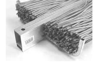
Picture shows 12" wide Cent-R-Rail cable tray with 3" load depth. The tray contains 520 4 UTP Category 5 cables (.21" OD).
