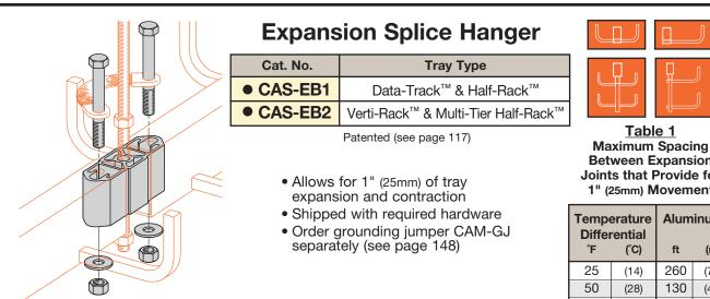
It is important that thermal contraction and expansion be considered when installing cable tray systems. The length of the straight cable tray runs and the temperature differential govern the number of expansion splice plates required (See Table 1).
