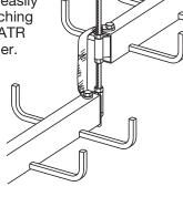
Note: Bonding jumper is required to maintain electrical continuity. (pg. 148)
