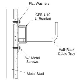
Note: These mounting details serve as a vertical support, and can serve as seismic bracing. See the Cent-R-Rail Seismic Restraints brochure for details.
