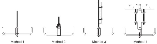
Method 1: 1/2" ATR passing through splice hangers (CAS-SB) with hex nuts on top and bottom.
