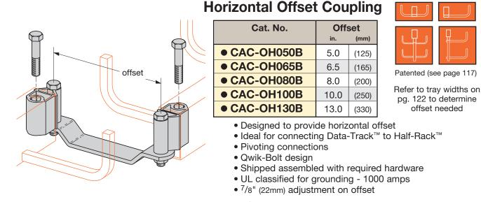
Note: All connectors are aluminum material and sized for 1/2" zinc plated steel hardware, unless otherwise specified.
