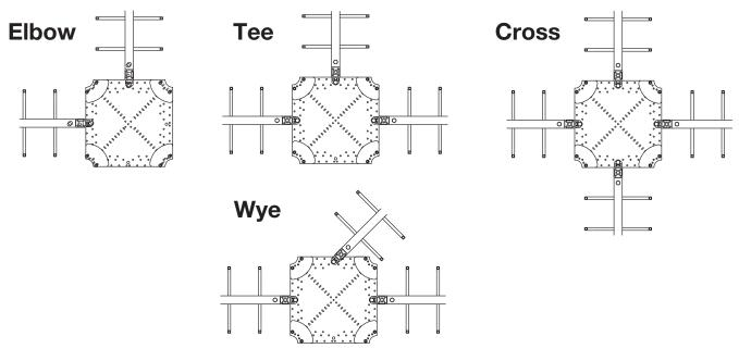
Note: All connectors are aluminum material and sized for 1/2" zinc plated steel hardware, unless otherwise specified.
