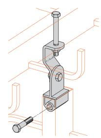
Note: All connectors are aluminum material and sized for 1/2" zinc plated steel hardware, unless otherwise specified.
